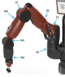
Fig. 1. Seven-DOF Baxter's arm at DSCL.
