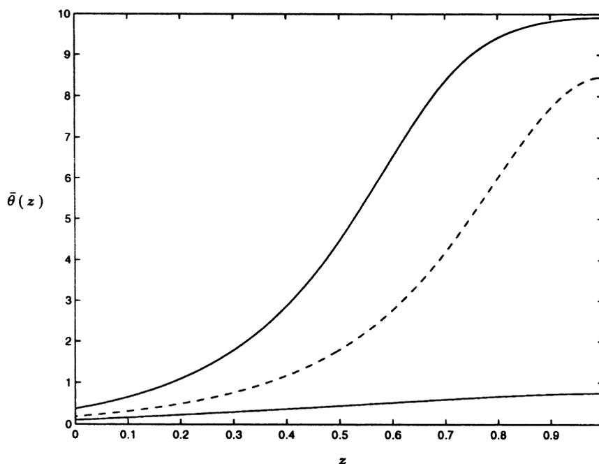
Fig. 1. Steady state temperature profiles for the adiabatic chemical tubular reactor with  $Pe_\theta = Pe_y = 6$ ,  $Da = 0.05$ ,  $\varepsilon = 0.05$ , and  $B = 10$ .
