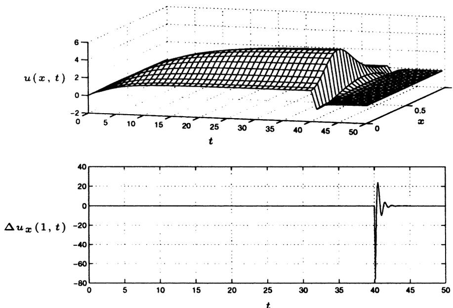
Fig. 2. Closed-loop temperature response with controller designed for  $N_c = 2$ ,  $C_1 = 3.5$ , and  $C_2 = 5$  (first row,  $u(x, t)$ ; second row, the control effort  $\Delta u_x(1, t)$ ).
