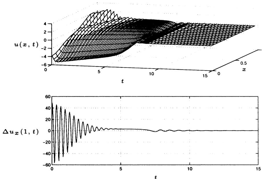
Fig. 4. Closed-loop temperature response with controller designed for  $N_c = 3$ ,  $C_1 = 5$ , and  $C_2 = 2.5$  (first row,  $u(x, t)$ ; second row, the control effort  $\Delta u_x(1, t)$ ).
