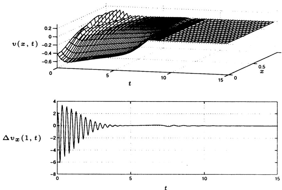
Fig. 5. Closed-loop concentration response with controller designed for  $N_c = 3$ ,  $C_1 = 5$  and  $C_2 = 2.5$  (first row,  $v(x, t)$ ; second row, the control effort  $\Delta v_x(1, t)$ ).
