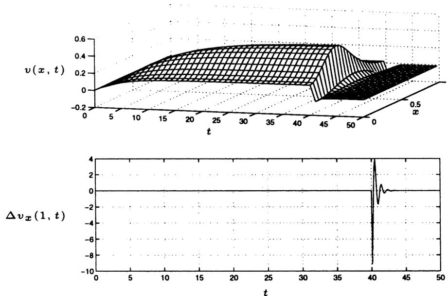
Fig. 3. Closed-loop concentration response with controller designed for  $N_c = 2$ ,  $C_1 = 3.5$ , and  $C_2 = 5$  (first row,  $v(x, t)$ ; second row, the control effort  $\Delta v_x(1, t)$ ).
