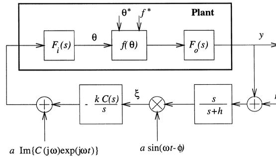
Fig. 1. Implementation of the extremum seeking algorithm with compensation.
