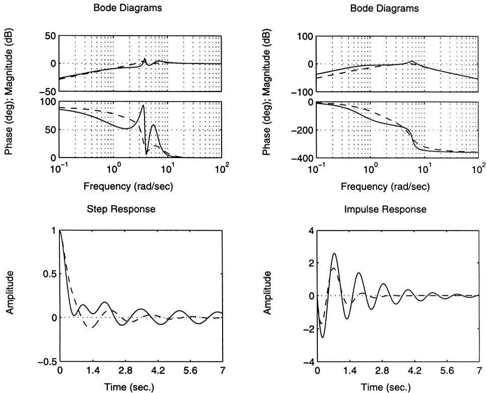
Fig. 6. Results for  $\tau=0$  and  $h=1$  (solid) and  $h=5$  (dashed). The plots on the left correspond to the transfer function  $1/(1+L(s))$  and the plots on the right are for the transfer function  $-M(s)/(1+M(s))$ .
