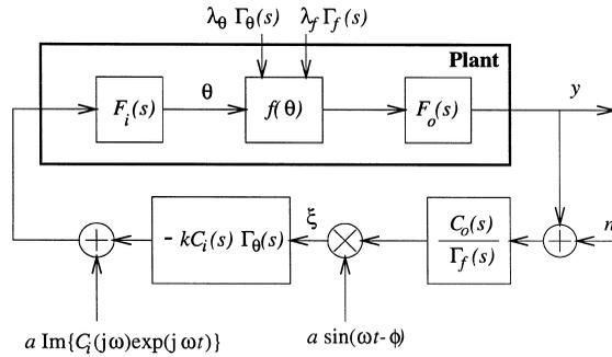
Fig. 3. Extension of the extremum seeking algorithm to non-step changes in  $\theta^*$  and  $f^*$ .
