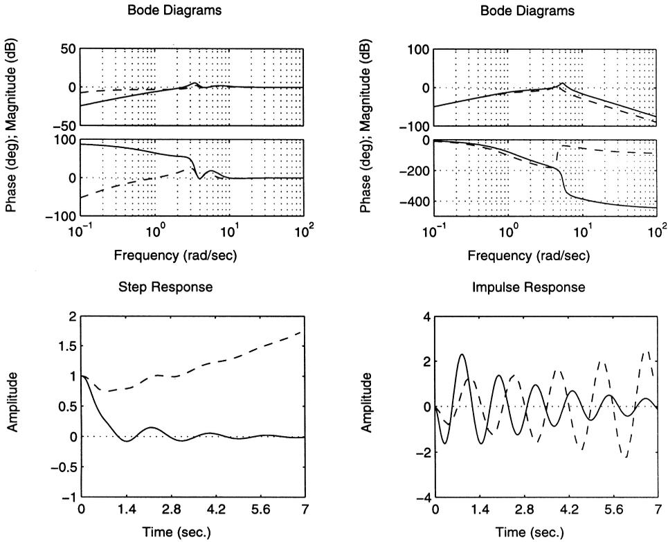
Fig. 7. Results for  $\tau = 0.12$  (solid) and  $\tau = 0.6$  (dashed). The plots on the left correspond to the transfer function  $1/(1 + L(s))$  and the plots on the right are for the transfer function  $-M(s)/(1 + M(s))$ .
