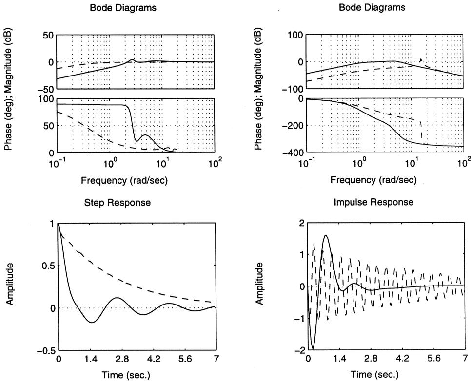
Fig. 5. Results for  $\tau = 0$  and  $\omega = 3$  (solid) and  $\omega = 15$  (dashed). The plots on the left correspond to the transfer function  $1/(1+L(s))$  and the plots on the right are for the transfer function  $-M(s)/(1+M(s))$ .
