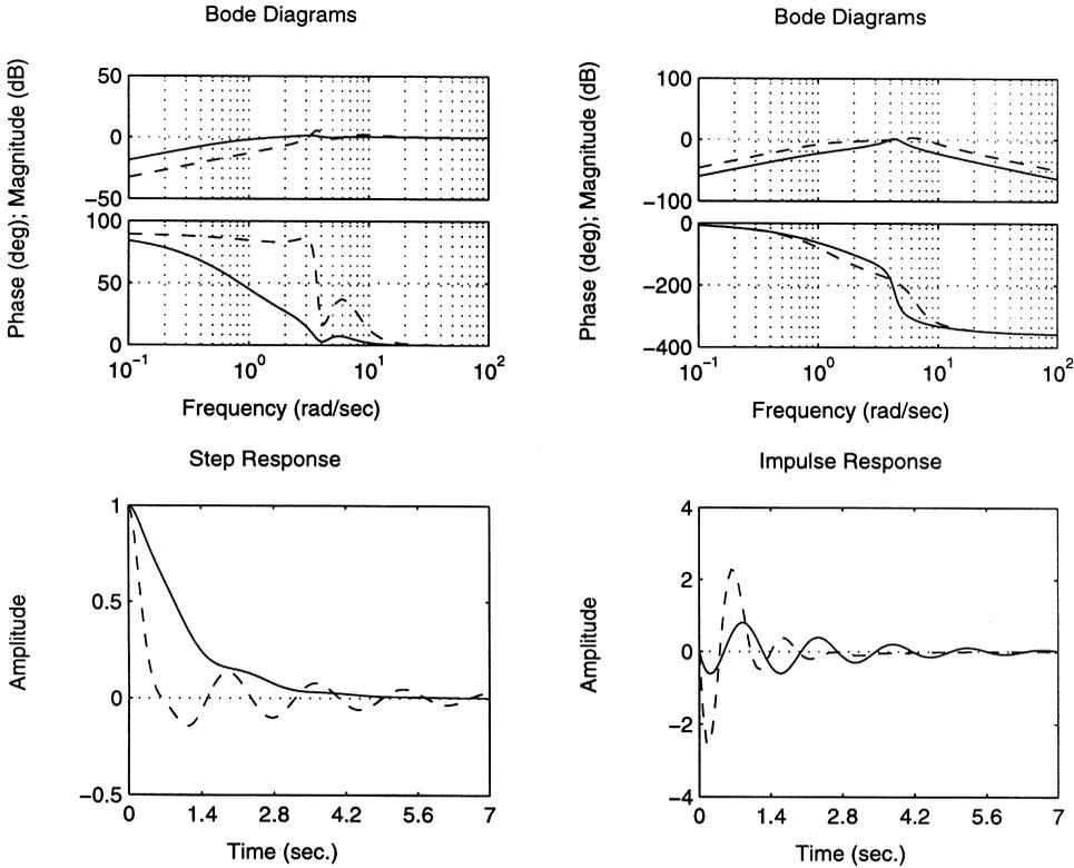
Fig. 4. Results for  $\tau = 0$  and  $q = 3$  (solid) and  $q = 15$  (dashed). The plots on the left correspond to the transfer function  $1/(1 + L(s))$  and the plots on the right are for the transfer function  $-M(s)/(1 + M(s))$ .
