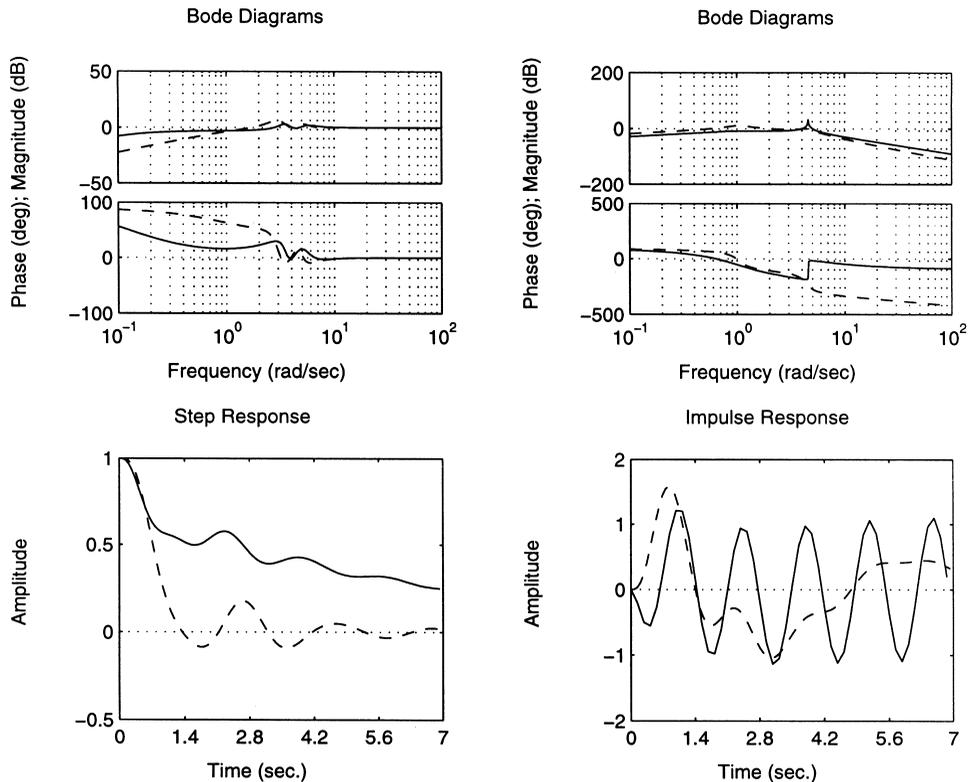
Fig. 9. Results for  $\tau=0.6$  and  $\phi=0.3$  (solid) and  $\phi=1.5$  (dashed). The plots on the left correspond to the transfer function  $1/(1+L(s))$  and the plots on the right are for the transfer function  $-M(s)/(1+M(s))$ .
