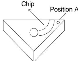
Fig. 1 Tool temperature measurement position (A) by infrared pyrometer
