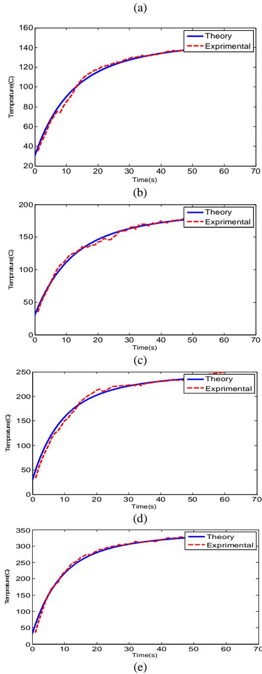
Fig. 2. Tool temperature vs. Time in (a)  $V=131$  mm/s, (b)  $V=185$  mm/s, (c)  $V=263$  mm/s (d)  $V=528$  mm/s and (e)  $V=733$  mm/s
