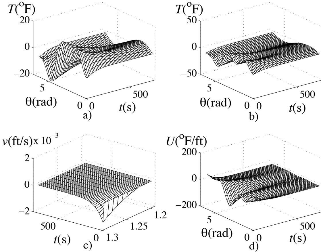
Fig. 4. Closed loop simulation. a) temperature at radius  $r = 1.21$  ft. b) temperature at radius  $r = 1.25$  ft. c) velocity d) temperature control effort
