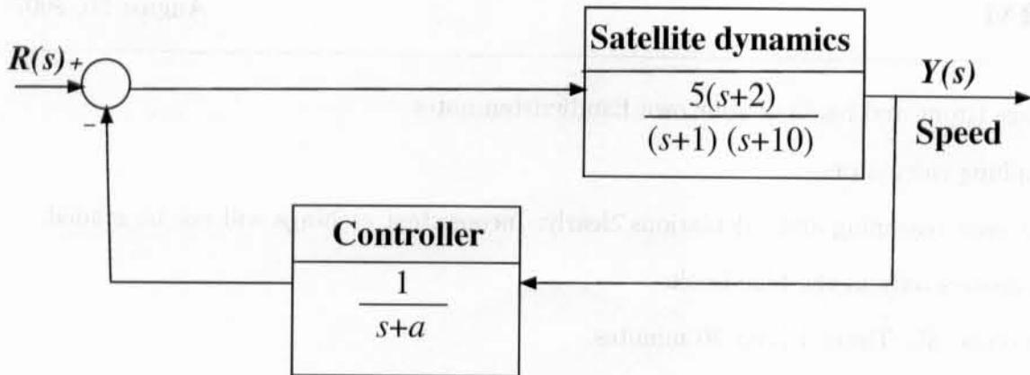
Find the sensitivity of the closed-loop transfer function  $T(s)$  to a small change in the parameter  $a$ .
