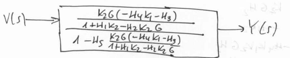
$$\frac{Y(s)}{V(s)} = \frac{-k_2 G (H_4 k_1 + H_3)}{1 + H_1 k_2 - H_2 k_2 G + H_5 k_2 G (H_4 k_1 + H_3)}$$
