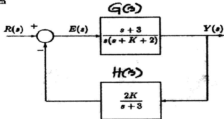
(a) (2 points) Find the closed-loop and error transfer functions:
