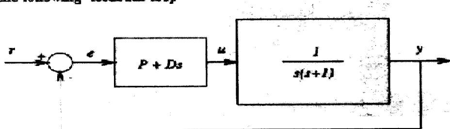
Find the values of the proportional gain  $P$  and the derivative gain  $D$  so that the rise time be  $t_r = 0.8$  seconds and the settling time be  $t_s = 2.3$  seconds.
