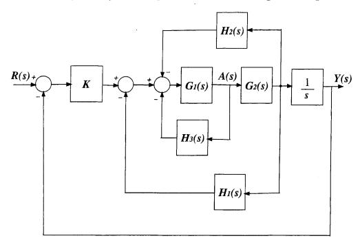
In the diagram, Y(s) is the ship's course, R(s) is the desired course (reference), and A(s) is the rudder angle. Find the transfer function Y(s)/R(s).
