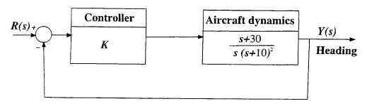
Determine the maximum gain K for stable operation.
