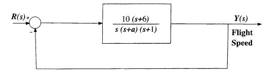
Find the sensitivity of the closed-loop transfer function T(s) to a small change in the parameter a.
