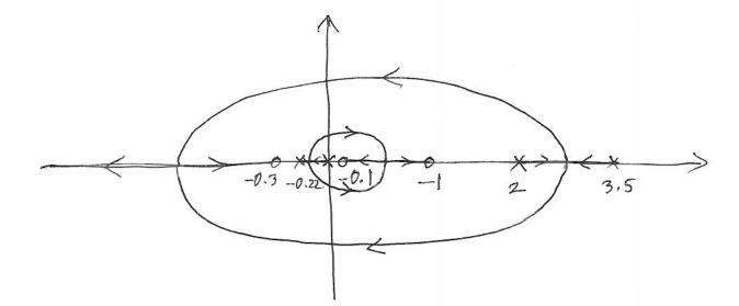
This is one of the many possible speculative solutions that happens to actually work. The stabilizing range for K is (5.52, 5.96).
