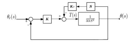
(b)(2 points)Use the block diagram to find the transfer function  $G(s) = \frac{\theta}{\theta_r}$  (You must do (a) first).
