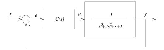
Find the parameters of a PID controller
