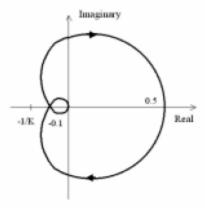
For positive K, note that the magnitude of the Nyquist plot as it crosses the negative real axis is 0.1, hence K < 10 for stability. For negative K, the entire Nyquist plot is essentially flipped about the imaginary axis, thus the magnitude where it crosses the negative real axis will be 0.5 and the stability limit is that |K| < 2 Therefore, the range of K for stability is -2 < K < 10.
