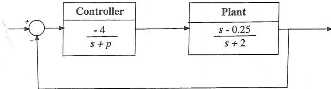
Using the idea from the beginning of the lecture notes on Root Locus, sketch the variation of the closed-loop poles as the controller pole  $p$  varies from 0 to  $+\infty$ .
