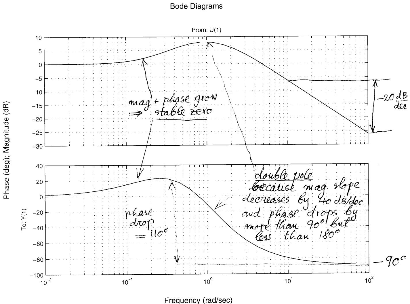
If this system has only *stable, real* poles and zeros, what is the minimum number of poles and zeros sufficient to produce this frequency response (choose one; answers without justification will not receive credit even if they happen to be correct):
