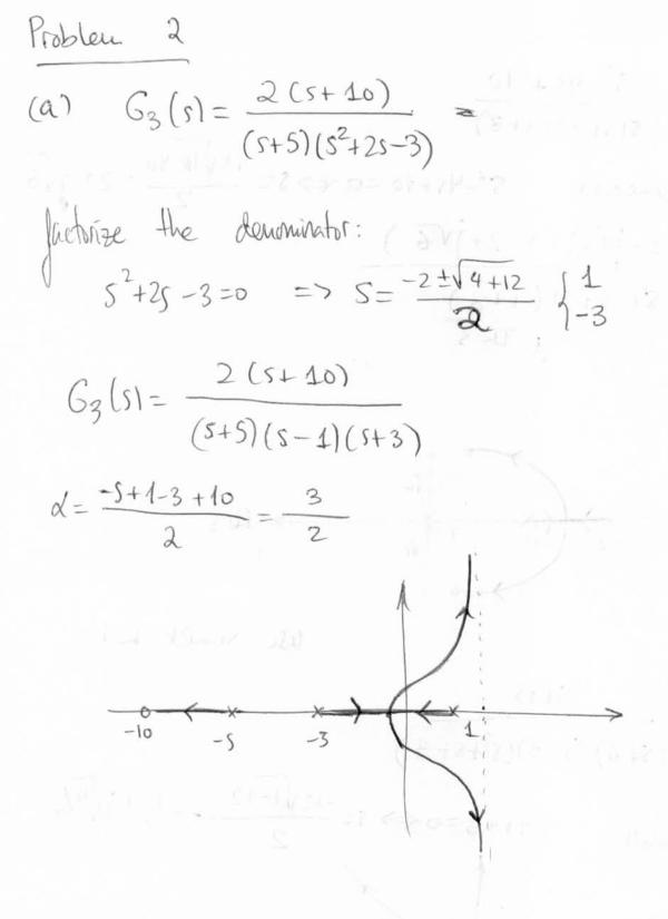
outy flok can make the system a.s. or not (but large sain does not work for sure) Check with Routh's criterion with K=1:  $T(s) = \frac{G_3(s)}{1 + G_3(s)} = \frac{2(s+10)}{(s+s)(s^2+2s-3)+2(s+10)} = \frac{2(s+10)}{s^3+7s^2+9s+5}$
