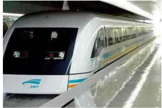
Figure 2. The high-speed, Chinese-Transrapid EMS-type MagLev train.
