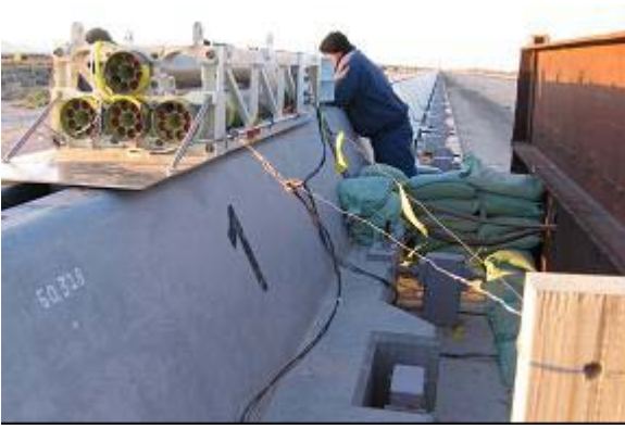
Figure 11. Sled with 4 HVAR motors installed
