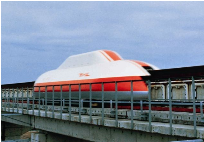
Figure 1. The first test vehicle on the Miyazaki Test Track "ML-500" recorded 517 km/h in 1979.
