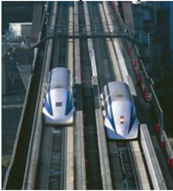
Figure 4. In the high-speed passing tests, relative speed of 1,003 km/h was recorded in 1999.
