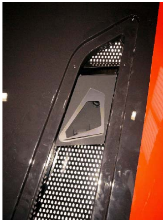
Figure 11. Camera system integrated in the front lights
